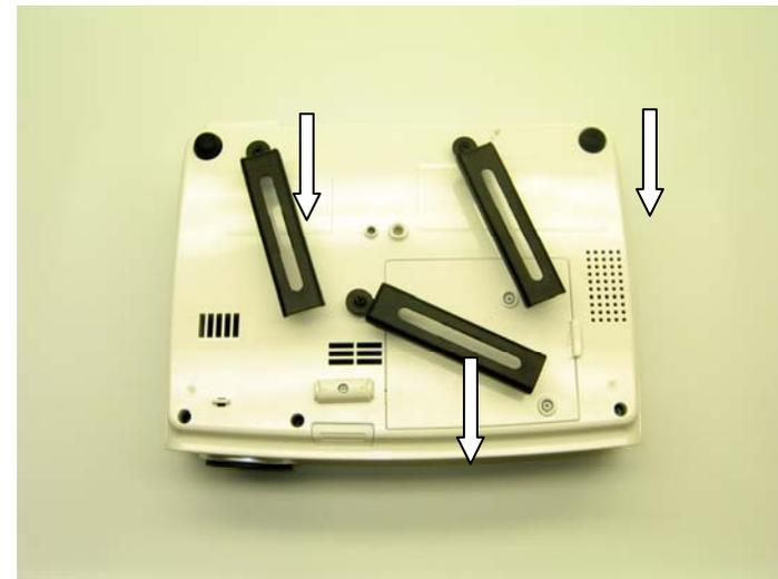
Take the LFM-style projector mount and place it on top of the mounting brackets. You may need to adjust your mounting brackets so they fit on the LFM-style projector mount.
