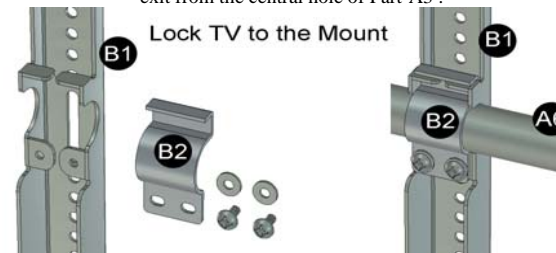
Figure 10: Lock Part-B to Part A
